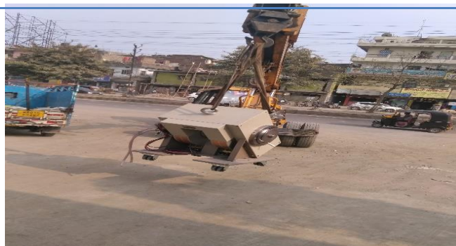
EQUIPMENT SHIFTING THROUGH JCB/Forklift
